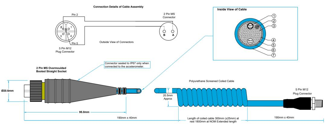
Environment Specification of Cable Assembly Maximum operating temperature of 150°C with high levels of resistance to chemical attack.
