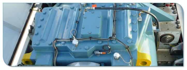
Secondly, accelerometers should then be correctly mounted – close to the component being monitored, on a flat, clean surface to guarantee consistent results. Poor mounting reduces reliability and can make collected data redundant – which means a machine might break down without warning even though it seems healthy and in fine working order.
