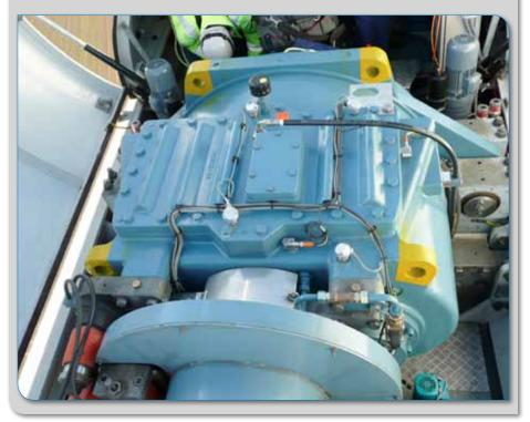
There are two main categories: AC accelerometers, which are used with a data collector for monitoring the condition of higher value assets, and 4-20mA accelerometers, which are used with a PLC to measure lower value assets. Both are capable of detecting imbalance, bearing condition and misalignment but AC accelerometers can also identify cavitation, looseness, gear defects and belt problems.
